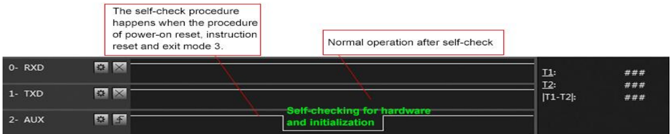
Timing Sequence Diagram of AUX when self-check
